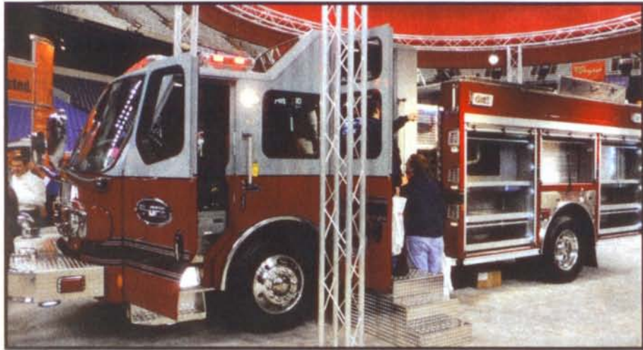
E-ONE exhibited a custom cab and chassis pumper with top-mount controls and an enclosed pump panel. The unit also featured a trimmed down pump module to shorten the overall length and increase maneuverability.
