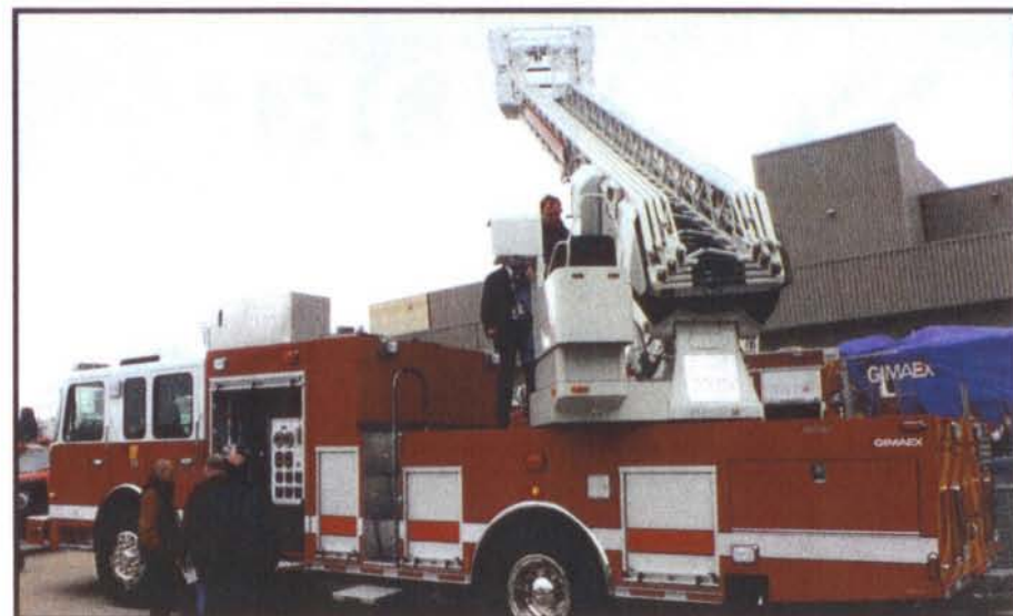
Gimaex demonstrated its unique platform aerial at FDIC this year. The apparatus is built on a Spartan cab and chassis and features a controller's seat on the turntable. (Fire Apparatus Photos by Ed Ballam)
